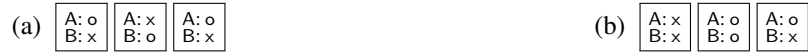
Figure 2: Two ways of voting for the second candidate (candidate B) in the ThreeBallot protocol, where x represents a marked position and o represents an unmarked position. All other ways of voting for B can be obtained as permutations of these two.
