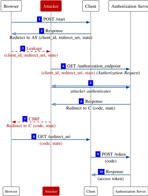
**Figure 7.** Leakage of Authorization Request Attack
