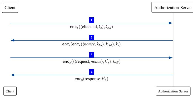
**Figure 9.** Detailed view on mTLS
